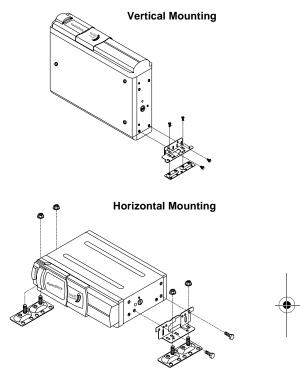
1. Set **SPRING ATTACHMENT H/V** (horizontal/vertical) on both sides of the CD changer for the mounting axis you chose.
